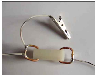
Figure 2— The band switches are constructed from nylon spacers, some wire and an alligator clip.
